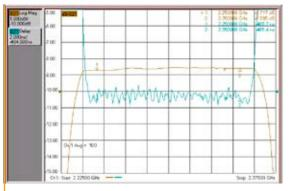
figure 5: IZT C3040 gain and group delay flatness
