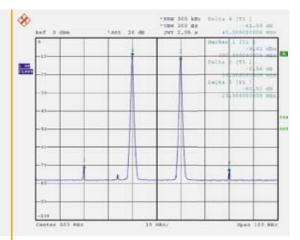
figure 15: IZT C3040 third order intermodulation products
