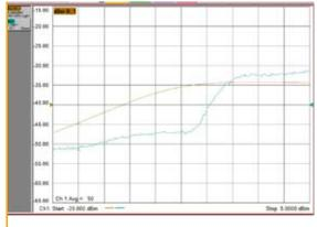
figure 10: Emulation of payload nonlinearity
