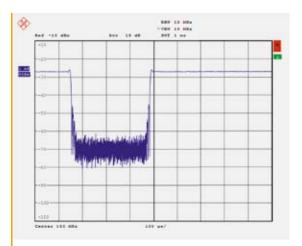
figure 12: Signal drop-out simulated with fast fading option
