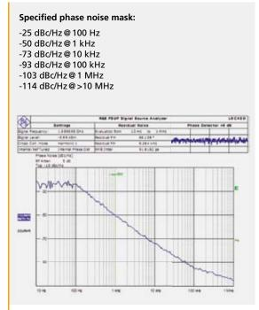
figure 9: Simulated phase noise "DVB-S2 typical"
