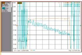
figure 6: Emulation of the ionosphere with IZT C3040
