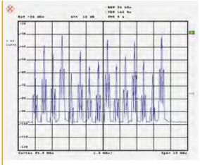
figure 12: Fifteen HD Radio signals
