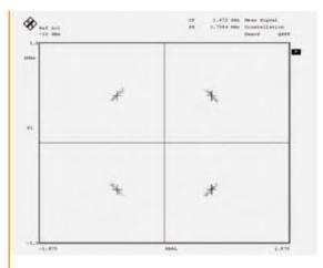
figure 9: QPSK constellation affected by phase noise
