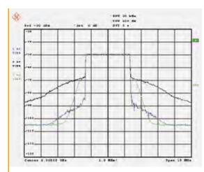
**figure 8:** Distorted signal before (black), after the filter simulation (green) and after filter simulation with alternative filter settings (blue).
