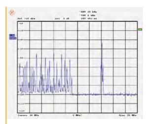
**figure 10:** Recorded FM broadcast spectrum combined with one HD Radio signal
