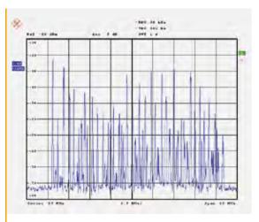
figure 5: Recorded FM broadcast spectrum
