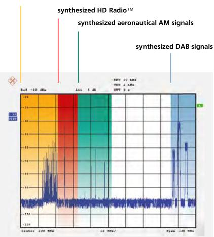
figure 2: Synthesizing a spectrum with the IZT S1000 over its full bandwidth
