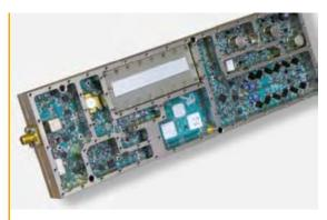
figure 3: RF section of the IZT \$1000
