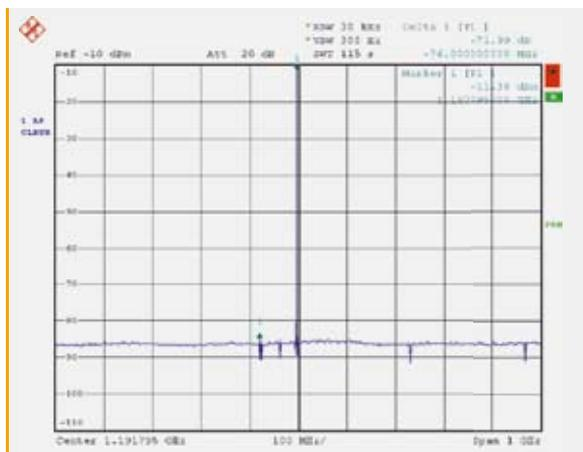
figure 14: Excellent spurious performance and signal-to-noise ratio
