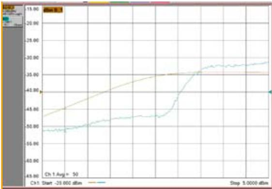
figure 10: Emulation of payload nonlinearity
