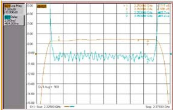
figure 5: IZT C3040 gain and group delay flatness
