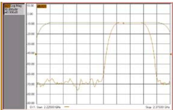
figure 7: IMUX and OMUX filtering
