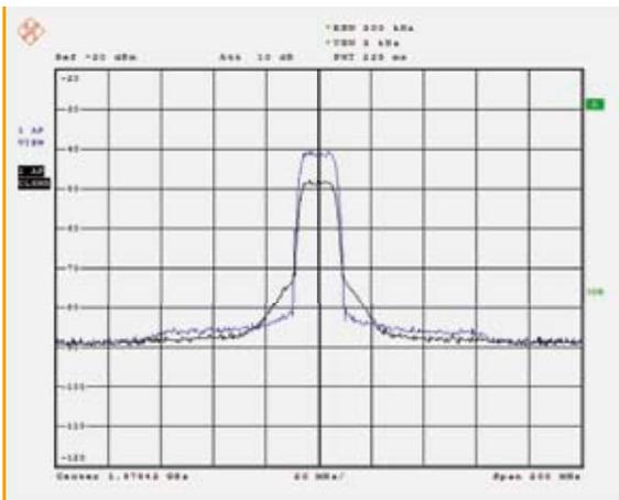
figure 11: Nonlinearity simulation with a QAM signal
