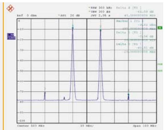
figure 15: IZT C3040 third order intermodulation products
