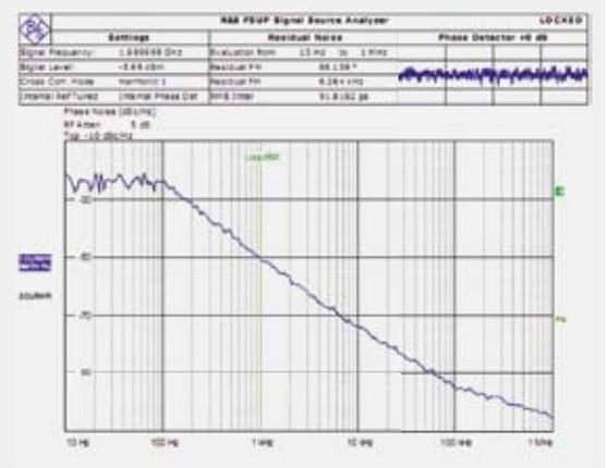
figure 9: Simulated phase noise "DVB-S2 typical"
